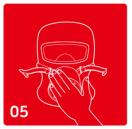
Inhale deeply while blocking the filter with your hand to check the gas-tightness.
